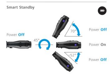
When Smart Standby is enabled, the device automatically switches to power-saving mode when you tilt it up more than 70° or down more than 52.5°. If you place your thermal imaging camera on an edge when not in use while up on your raised hide, it automatically switches to intelligent standby mode – at a 45° angle to the left or right.
