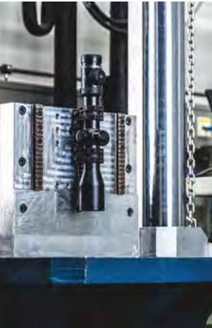
Testing extreme situations: significant temperature fluctuations within minutes and shot simulations with 1,500 times the force of gravity.
